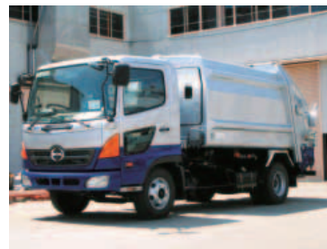
Refuse collection vehicle equipped with a body weighing system
