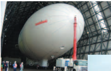
68-meter model coming out of the hangar (The front truck is called a mast car)
