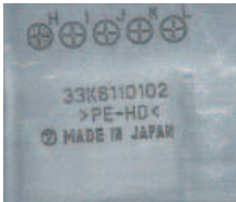
Resin part that indicates its material sign
