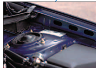
Shock absorbing Structures are built into the upper parts of fenders.
