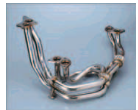
Equal length/constant pulsation independent exhaust manifolds
