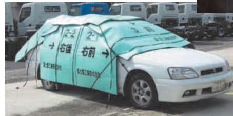
When sound arresting sheets are installed
