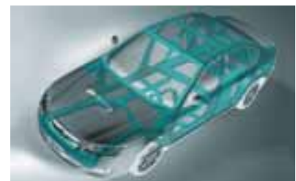
The new ring-shaped reinforcement structure
