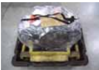
(Picture 5) SCI's returnable/reusable long-engine container
