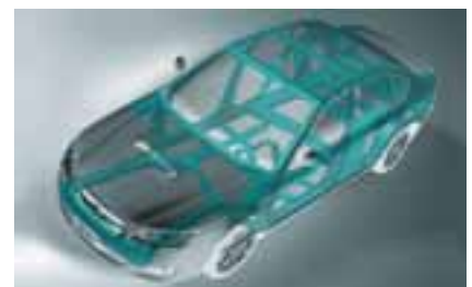
The new ring-shaped reinforcement structure
