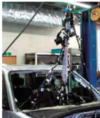
Picture 1 : Wire harness dismantling experiment
