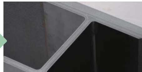
Example of a sectional view of a part formed by the autoclave Stacked layers of carbon fibers are visible.
