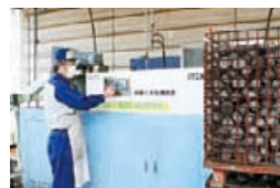
A Grinding sludge briquetting machine which has the both roles, one is wastes reduction and the other is making some profit.
