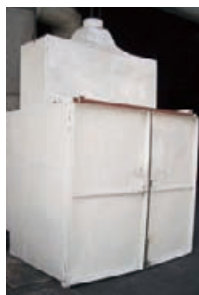
A sound-proof chamber for burr containers of Ichitan Co., Ltd.
