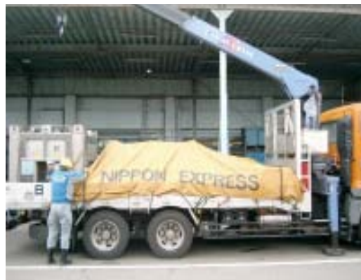
Loading PCB waste to a truck
