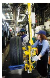
Power assist for tire fitting
