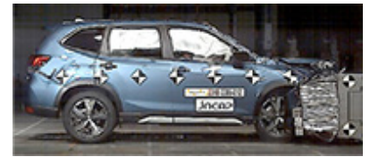
Image of Forester JNCAP* Frontal Offset Crash Test Source: National Agency for Automotive Safety & Victims’ Aid
